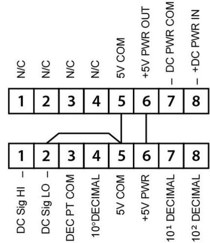
Figure 2 Wiring Diagram
