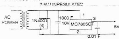
Figure 1. Typical Power Supply Schematic Diagram
